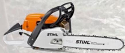
The additional QuickStop Super chain brake (Q), a STIHL exclusive, provides an added layer of safety. The saw chain not only stops in seconds whenever there is a sufficiently strong kickback or the front hand guard is activated, but also whenever the user lets go of the rear handgrip. A key benefit is that QuickStop Super operates in all working positions – without the need for an additional lever or handle.
