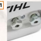
It's impossible to lose the sprocket cover nuts when you're swapping cutting attachments, as they are attached to the actual sprocket cover.
