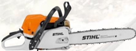
The electrically heated hand grip and carburettor (VW) makes your work more comfortable in the winter. The carburettor heating keeps the carburettor ready for use even in the cold, and prevents it from icing up in wintry conditions. The electric hand grip heating with on/off switch improves safety.
