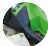
**Rubber bumper:** Front impact protector protects the machine and obstacles, can also be used as a carrying handle and for lashing
