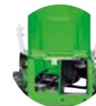
Easily accessible **service flap** at the rear for easy maintenance. Sturdy deflector flap with strong spring, suitable for rear discharge
