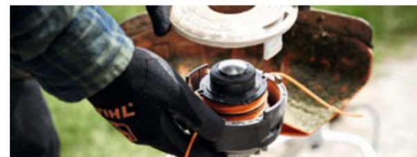
**AUTOCUT 27-2 MOWING HEAD AND SPOOL WITH METAL GUARD**
